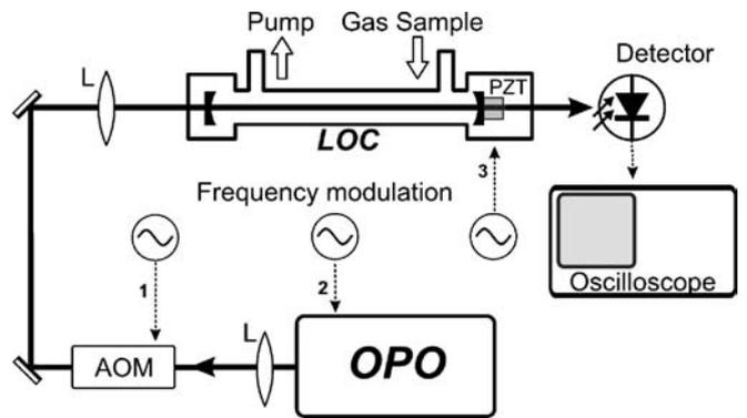
**FIGURE 8** Linewidth characterization setup using a ring-down cell (LOC). The cell is empty. Overlap between OPO emission and LOC resonance can be achieved by frequency modulation of the idler wave via the AOM (1) or, in the dual-cavity PR-SRO system, by modulating the signal cavity length (2), or by modulating the LOC length (3)
