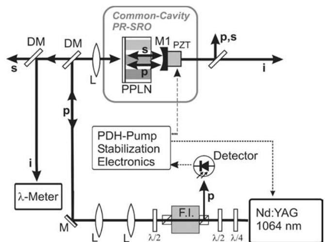
FIGURE 2 Common-cavity PR-SRO setup; M = mirror, DM = dichroic mirror, FI = Faraday isolator, L = lens, p = pump, s = signal, i = idler
