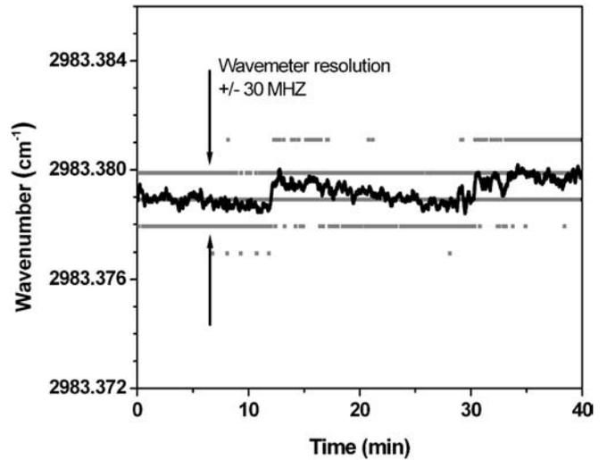
FIGURE 5 Long-term frequency stability (digital wavemeter read-out in 30 MHz steps and running average over 20 points) of the dual-cavity PR-SRO
