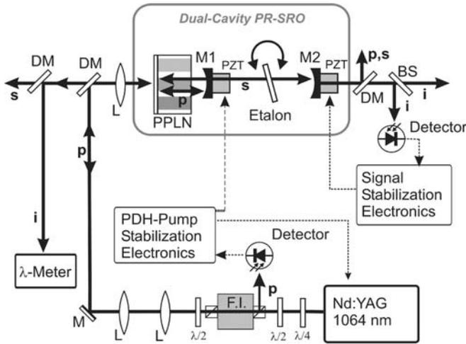
FIGURE 3 Dual-cavity PR-SRO; BS = beamsplitter
