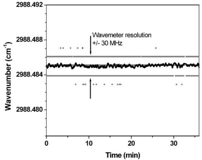
FIGURE 4 Long-term frequency stability (digital wavemeter read-out in 30 MHz steps and running average over 20 points) of the common-cavity PR-SRO
