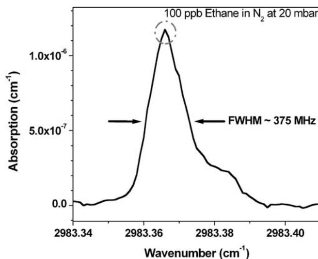
FIGURE 1 An ethane absorption structure at 20 mbar pressure obtained using CALOS and a dual-cavity PR-SRO. The gray circle marks the wavelength which is used for ethane monitoring
