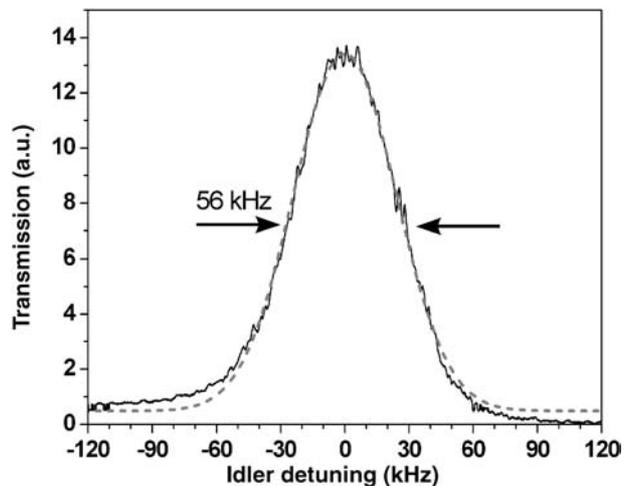
**FIGURE 9** Transmission of the common-cavity PR-SRO idler wave through the fixed-frequency LOC (solid line). Averaging time is 1.8 seconds (120 scans). Dashed line: Gaussian fit
