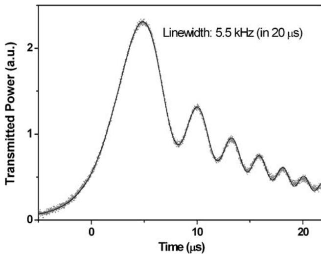
FIGURE 13 Measurement of the ringing signal (dots) and best fit (solid line) for the dual-cavity PR-SRO
