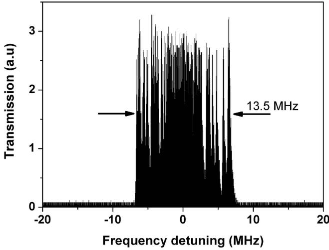
FIGURE 10 Transmission of dual-cavity PR-SRO idler radiation through the LOC, averaged over 1.5 seconds (100 scans)
