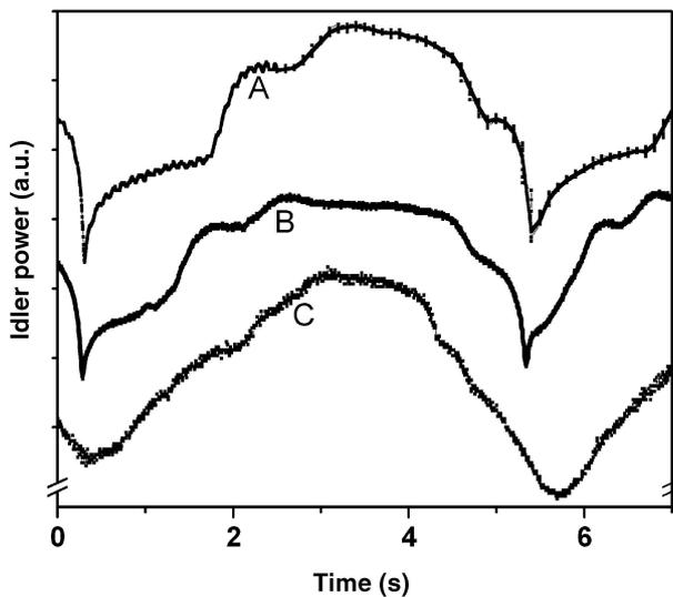
**FIGURE 7** Idler power measured while scanning the signal cavity length linearly in time over a little more than one FSR. Note that the time span is much less than in Fig. 6. Vertical shifts are introduced for a better visibility. Scan A is measured about 4 minutes after scan B, both showing clear structures. Scan C was measured about an hour later, showing less pronounced structures. The curves were shifted horizontally so that the positions of the mode-hops coincide
