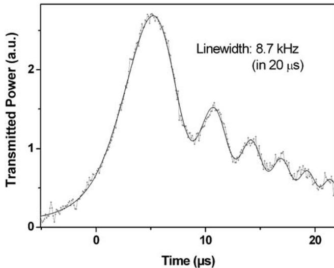
FIGURE 12 Measurement of the ringing signal (dots) and fit (solid line) for the common-cavity PR-SRO
