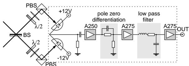
Fig. 1. Electro-optic scheme of the homodyne system.
