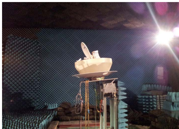
Figure A- 4 ACES MWL ground terminal under test in compensated compact range facility. The I-SOC-PF ground terminals will be based on the ACES technology.
