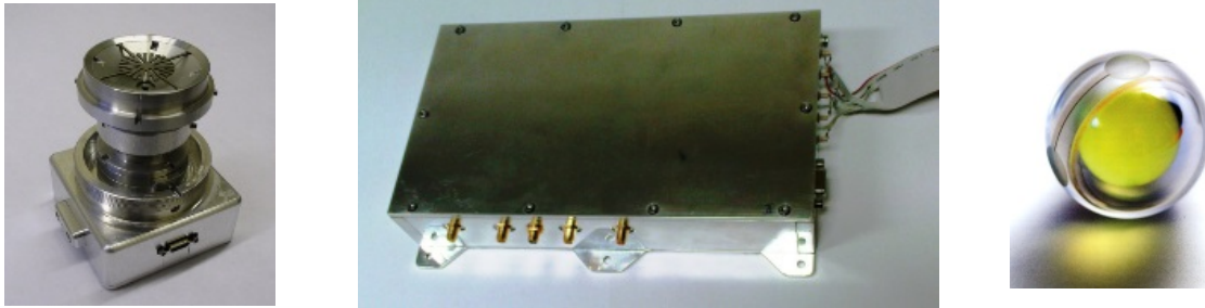
Figure A- 9 Left: Single-photon detector prototype. Center: Epoch (event) timing unit prototype. Right: Luneburg sphere (laser retroreflector).
