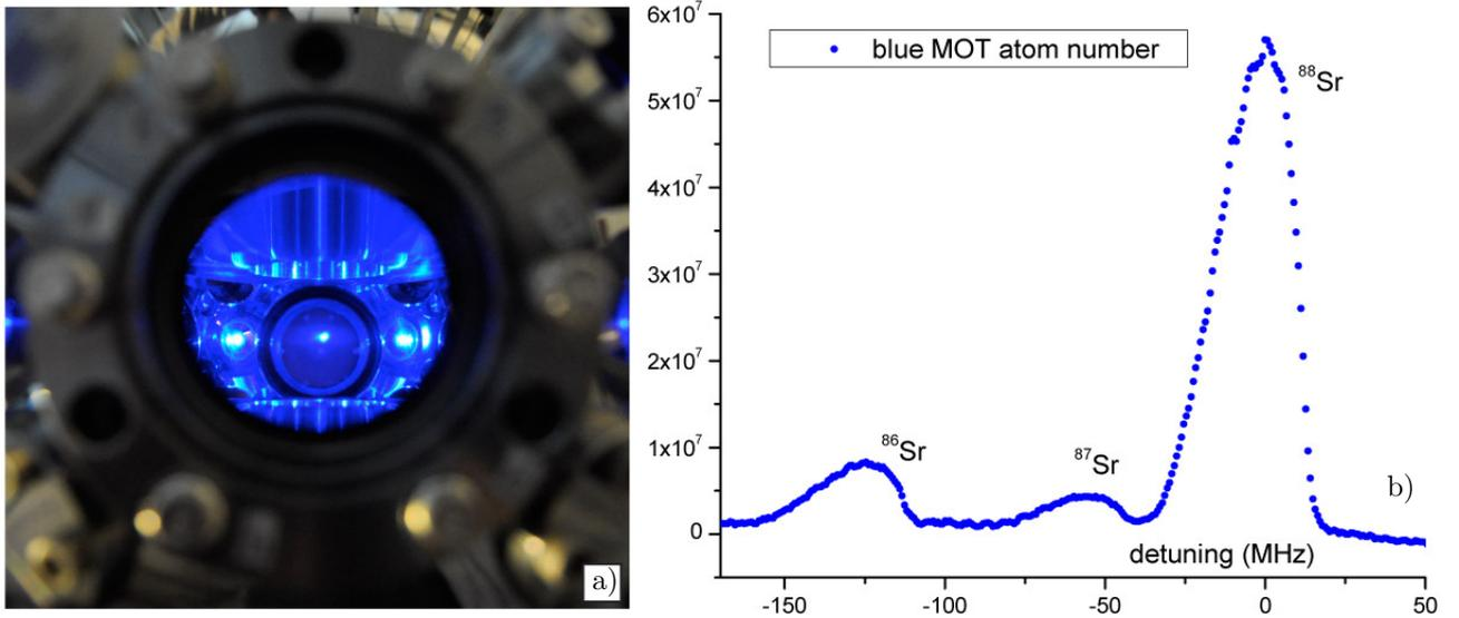
Figure 4: First magneto-optical trap (MOT) at 461 nm realized on the transportable setup. a) Picture of the  $^{88}\text{Sr}$  blue MOT seen by one of the CF40 windows used to collect the atom's fluorescence. b) Plot of the fluorescence signal in function of the blue laser detuning. Together with the signal due to the most abundant  $^{88}\text{Sr}$  (82.58%) also signals of  $^{87}\text{Sr}$  (7.00%) and  $^{86}\text{Sr}$  (9.86%) trapped atoms can be resolved.
