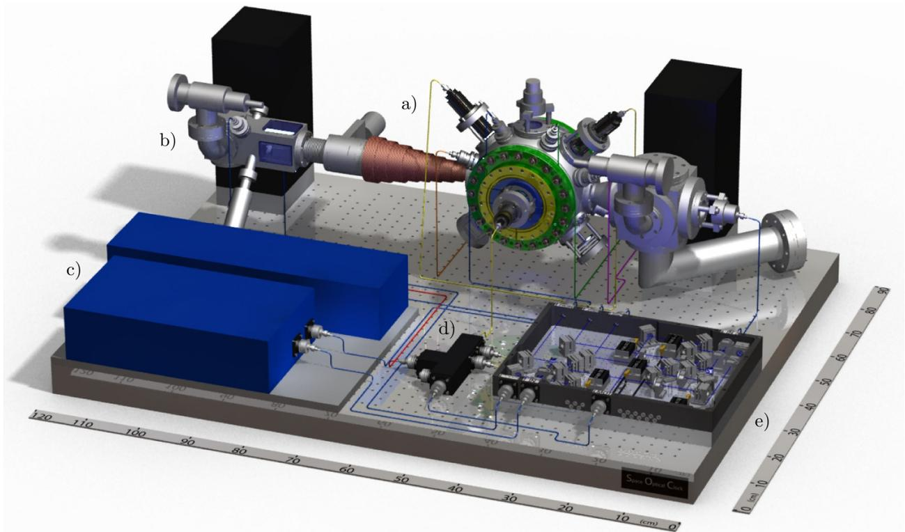
Figure 2: 3D model of the transportable cold strontium source. a) Vacuum system. b) High efficiency oven. c) Blue laser at 461 nm. d) Dichroic fiber port cluster. e) Compact breadboard for the opto-mechanics.
