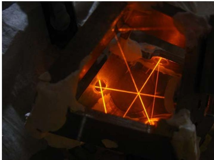
Fig. 5. Compact three-dimensional optical lattice for the Yb clock, formed by intersecting standing-wave laser beams (759 nm) in a folded optical cavity. The atom trapping region is at the three-fold intersection point. The beams were made visible by leaking water vapour into the vacuum chamber.
