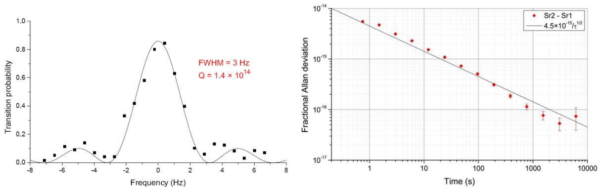
**Figure 1.** Left: Resonance line of ultracold Sr atoms at 698 nm in the optical lattice. The line has a quality-factor  $Q$  of  $1.4 \times 10^{14}$ . Right: Instability of the Sr optical clock pair, dropping to less than  $1 \times 10^{-16}$  (Observatoire de Paris).
