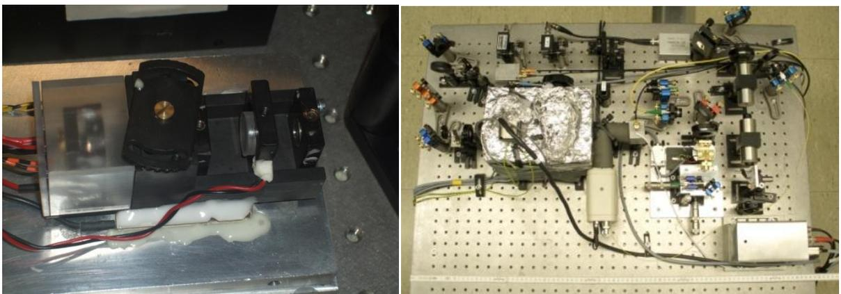
**Figure 5.** Left: Compact interference filter stabilized diode laser at 399 nm (power up to 40 mW,  $\sim 1$  MHz linewidth,  $\sim 300$  MHz tuning range, improved stability vs. grating ECDL). Right: Yb clock laser system. At bottom right is the 1156 nm diode laser, which is frequency doubled in a waveguide. Silvery box contains the ULE cavity (Universität Düsseldorf).
