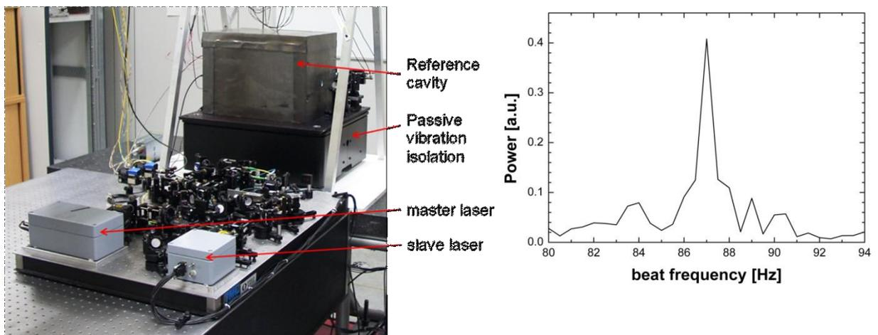
**Figure 3:** Left: Transportable clock laser for Sr interrogation (PTB Braunschweig). Right: Beat spectrum between the transportable laser (698 nm) and the clock laser for Yb (578 nm), after transport of the Sr clock laser from Braunschweig to Düsseldorf, obtained using a frequency-comb. The combined linewidth is at the 1 Hz level. Measurement time: 2 s; resolution: 0.5 Hz.
