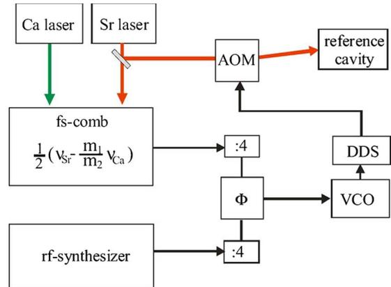
Fig. 6. Schematic of the phase lock of the 698-nm Sr laser to the 657-nm Ca laser serving as a reference.
