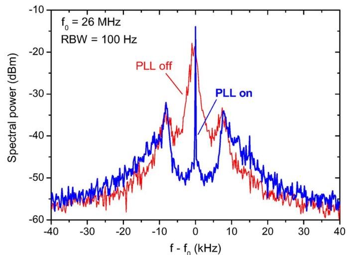
Fig. 7. Virtual beat between the Sr and Ca lasers with the PLL open and closed. With the PLL open, the noise of the free-running VCO is dominating. Both spectra are averaged over ten sweeps with a sweep time of 80 ms.
