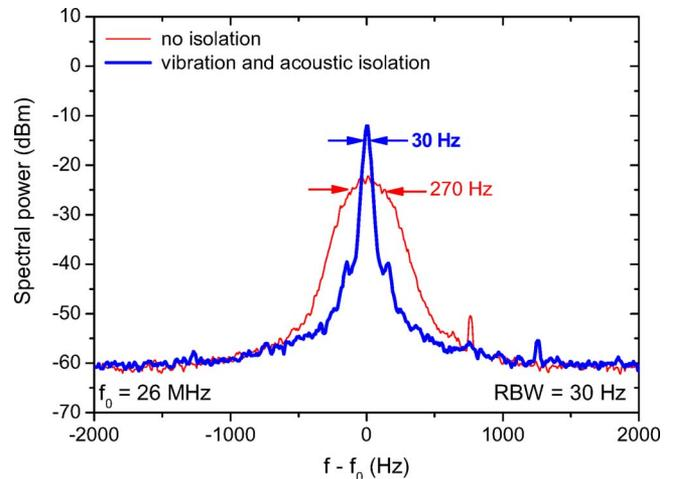
Fig. 3. Frequency spectrum of the virtual beat between the 698-nm Sr laser and the Ca reference laser. The spectrum obtained without any isolation (270-Hz linewidth) was averaged over ten sweeps of 0.135 s. The spectrum measured with a passive vibration isolation table and acoustic isolation (30-Hz linewidth) was averaged over 100 sweeps.
