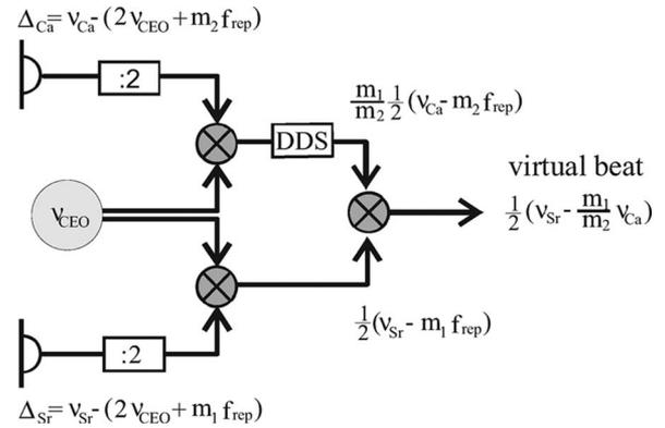
Fig. 2. Schematic of the RF electronics for generating a virtual beat signal between the strontium and the calcium laser. The fs comb acts as a transfer oscillator. Thus, the virtual beat is independent of the fluctuations of the repetition rate  $f_{rep}$  and the carrier envelope offset frequency  $\nu_{CEO}$  of the fs fiber comb.
