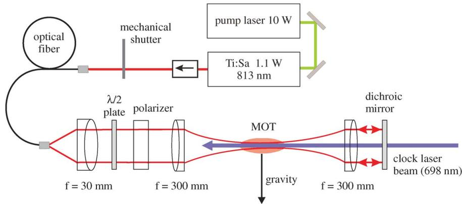
Fig. 4. Setup of the 1-D optical lattice at 813 nm. The 1-D lattice is directed perpendicular to gravity and to the axis of the MOT coils.
