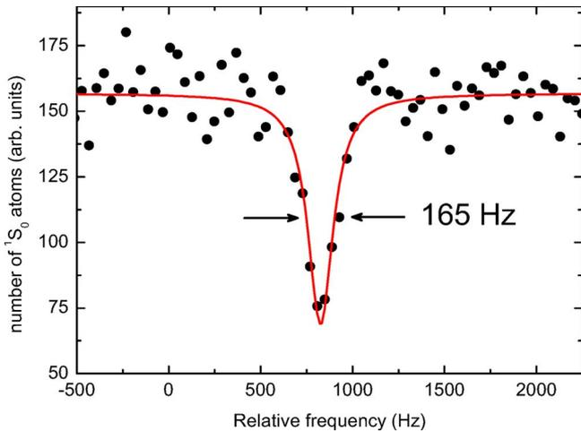
Fig. 5. Magnetically induced  $^1S_0-^3P_0$  clock transition of  $^{88}\text{Sr}$ . Each data point corresponds to a single measurement cycle of 640 ms. The frequency axis is determined from the offset between the reference cavity and the interrogation laser (twice the AOM frequency). It is corrected for the cavity drift and shifted by an arbitrary frequency to obtain small numbers.
